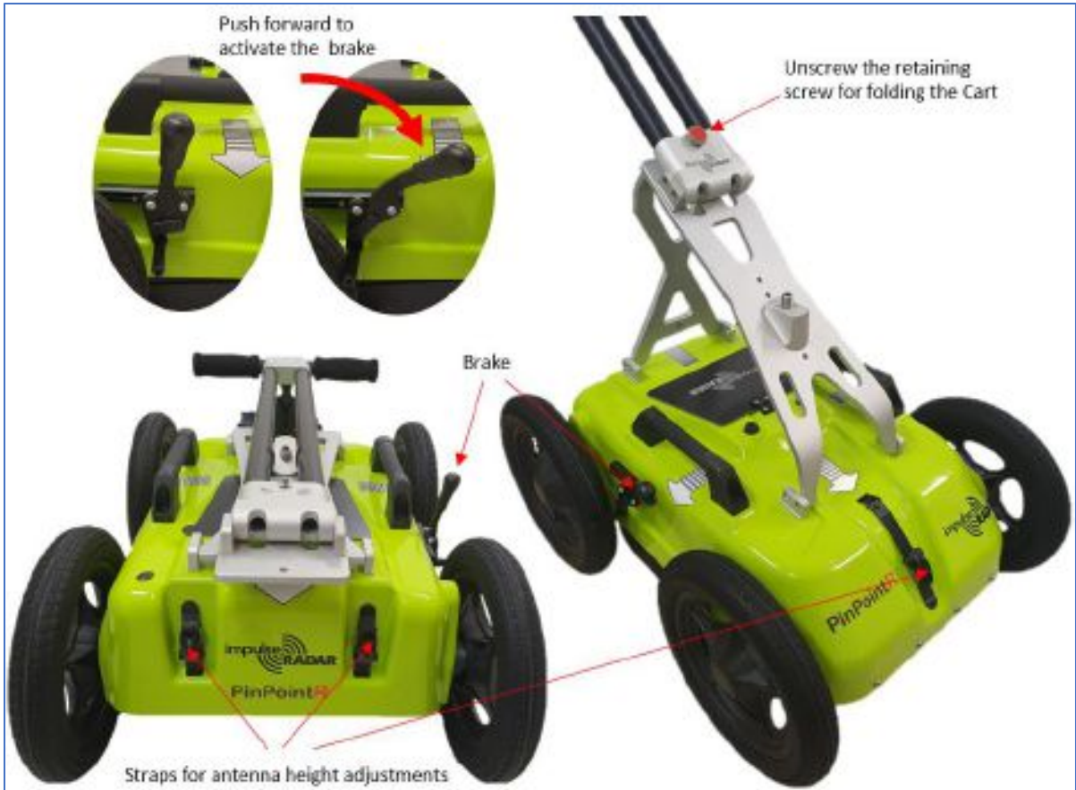
Figure 4 PinPointR push-cart features
