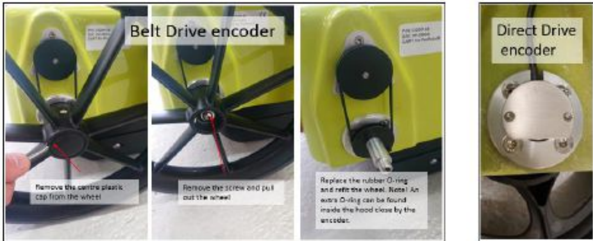
Figure 7 Belt or Direct Drive encoder and wheel assembly
