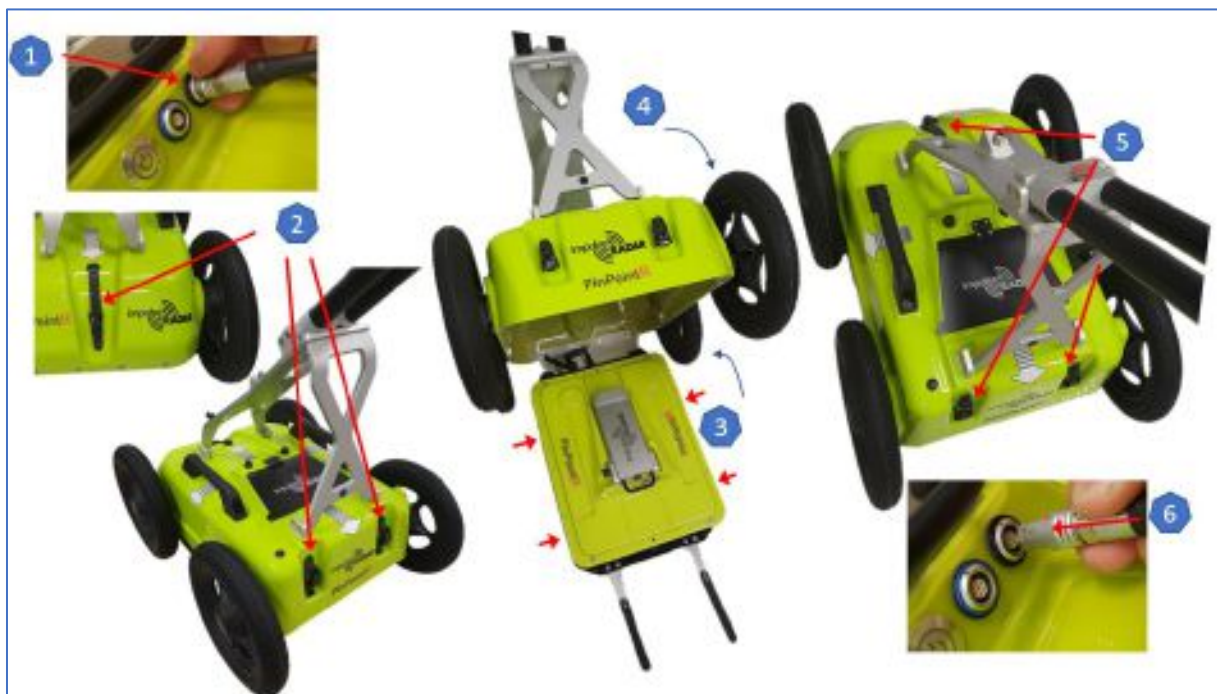
Figure 6 GPR unit fitting and height adjustments
